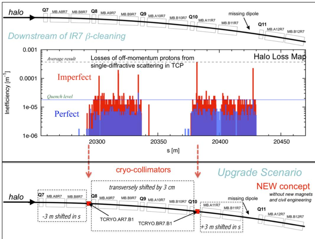
Figure 1: Illustration of present layout and proton losses (top) and proposed modified layout (bottom) in the dispersion suppressors around IR7 (betatron cleaning). Losses are given as local inefficiency and should be below the indicated quench limit for nominal intensity and nominal loss rate. Both the ideal loss map (blue bars, 40% intensity limit) and one typical imperfect loss map (red bars) are shown. Loss maps for ions are qualitatively different [4].
