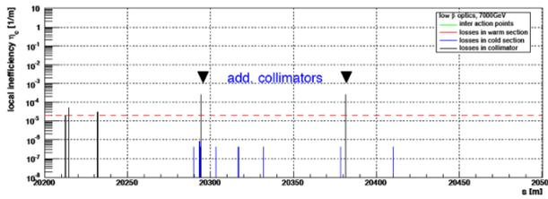
Figure 2: Proton losses (ideal local cleaning inefficiency) downstream of the IR7 betatron cleaning with the phase II system, nominal intensity and nominal peak loss rate on the primary collimator. Blue bars show losses in superconducting magnets, black bars losses at collimators.
