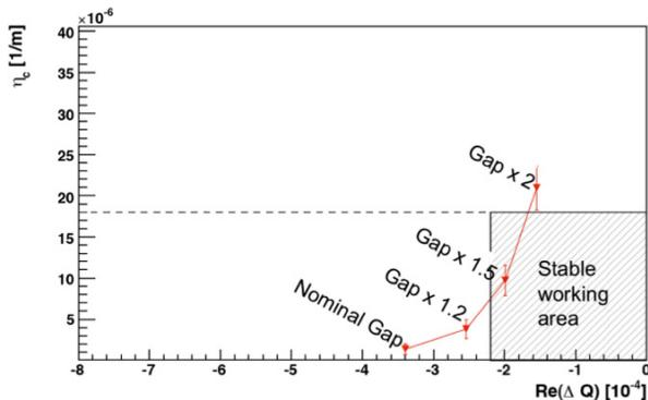
Figure 3: Inefficiency versus tune shift (impedance) for various collimation settings with gaps open. The stable working area for nominal intensity is shown.
