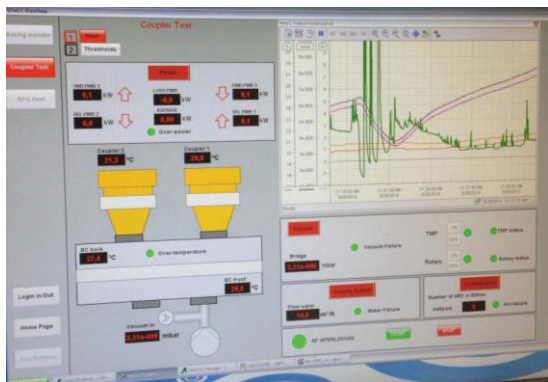
Figure 5: Screenshot of the Coupler High Power Test Data Acquisition System.
