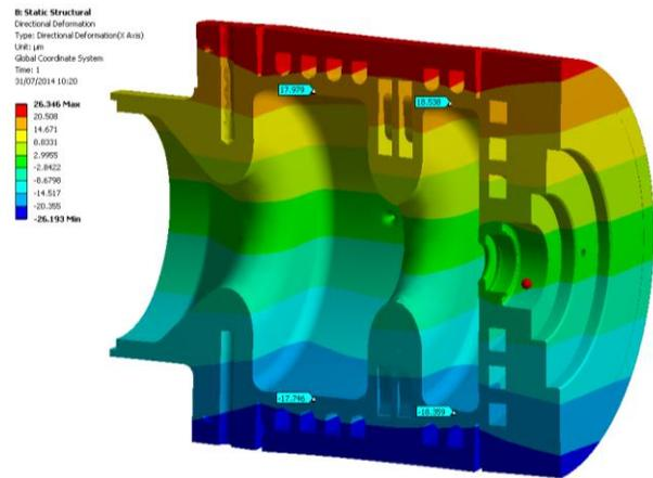
Figure 5: Radial cell deformation from room temperature to full operating temperature with RF.
