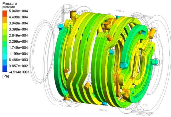
Figure 3: Pressure profile at the surface of the cooling channels.
