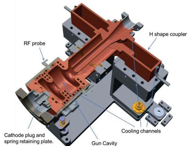
Figure 1: Overview of the gun cavity design.
