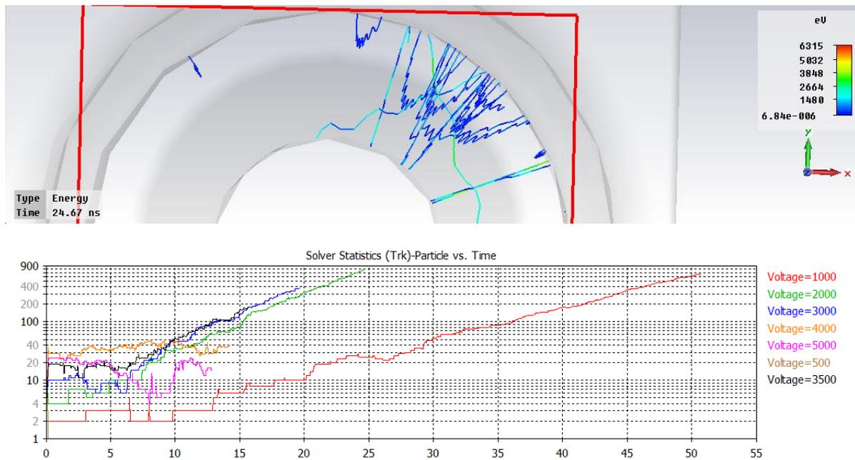
Figure 2: Multipacting trajectories in the coaxial coupler transition (top) and the number of electrons versus time at various voltages (bottom), RF power  $P$  is calculated as  $P=2V^2$ .
