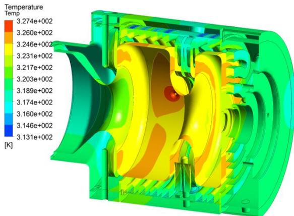
Figure 4: Temperature profile at the gun cavity surface.
