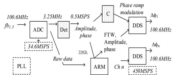
Figure 9: Simplified structure of the reference generator.
