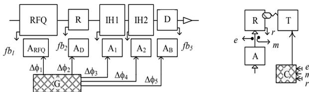
Figure 8: Structure of the HILAc LLRF system.
