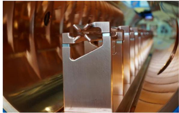
Figure 4: The 4 – Rod – RFQ during installation work.
