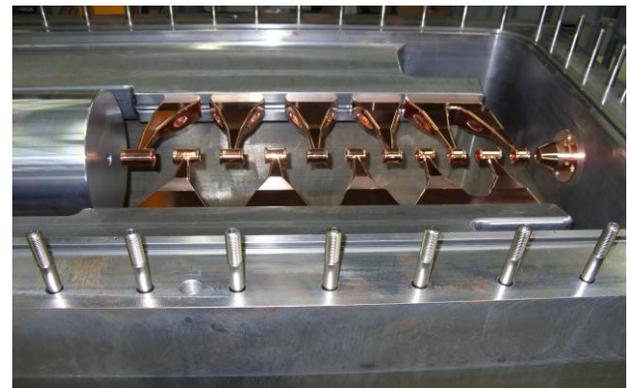
Figure 5: IH1 cavity prepared for first RF measurements.
