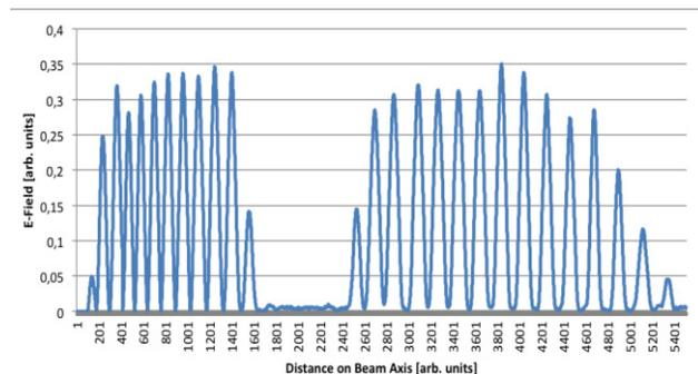
Figure 6: E - field distribution along the beam axis of cavity IH1.
