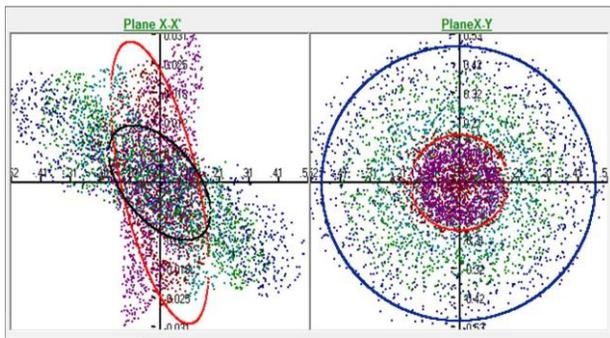
Figure 3: Phase plane and beam spot at RFQ entrance for 3.5 mA gold beam current with ions charge state spectrum from 29+ up to 32+ (different colors).
