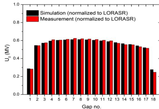
Figure 7: Gap voltage distribution along cavity IH2 and comparison with LORASR simulations
