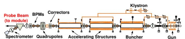
Figure 1: Layout of the CALIFES injector installed in CLEX.
