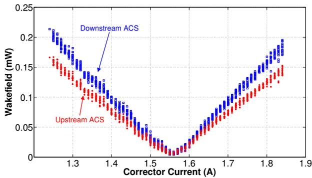
Figure 5: TE-like 24 GHz wakefield excited as function of the upstream vertical corrector current for the upstream (red) and downstream (blue) ACSs installed in TBTS.
