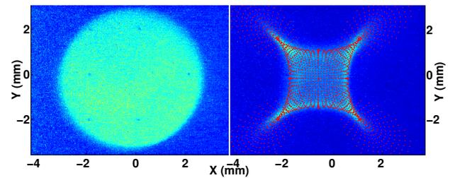
Figure 3: Transverse beam shape observed downstream the ACS without RF (left) and with 12 GHz RF at 306° phase (right).
