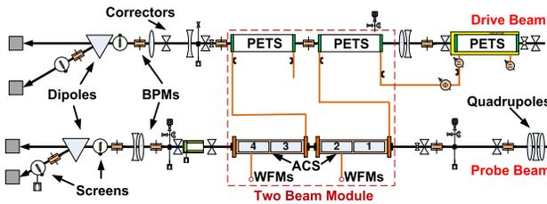
Figure 2: Layout of the module installation downstream the CALIFES injector.
