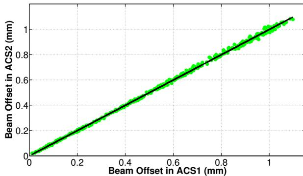
Figure 6: Correlation of measured beam position from 24 GHz excited wakefields (green dots) in downstream ACS with respect to position measured in upstream ACS and the expected lineal behaviour (black line).
