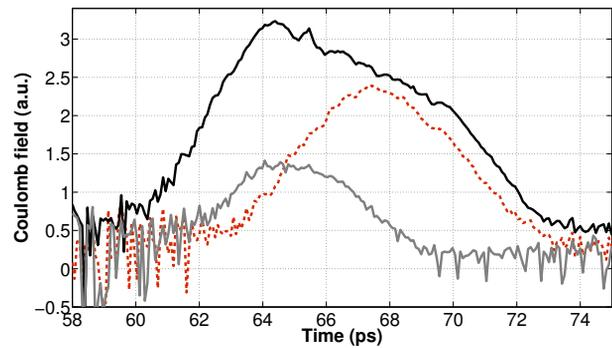
Figure 7: Temporal structure of the measured Coulomb field for 0.17 (grey solid), 0.3 (red dashed) and 0.7 nC (black solid) bunch charge.
