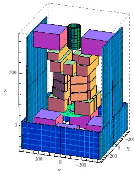
Figure 2: Layout of magnet and iron yoke.
