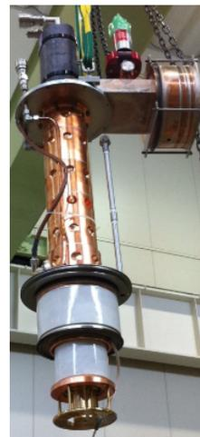
Figure 4: The klystron using in power test (Toshiba E37501).
