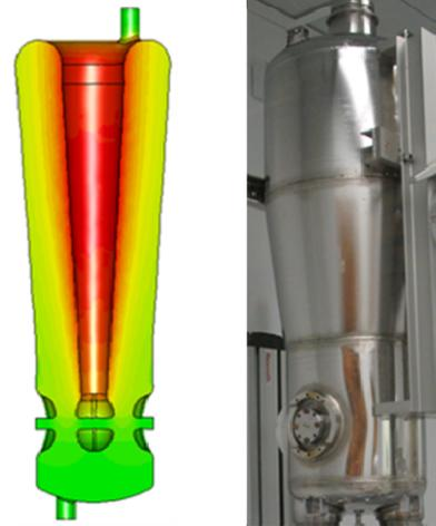
Figure 3: Cavity MWS model showing magnetic field distribution (left) and completed cavity assembly in the HPR apparatus (right).
