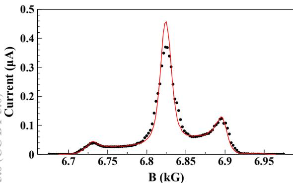
Figure 2: Measured (dots) and simulated (red curve) beam intensity as a function of the magnetic field.
