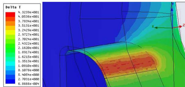
Figure 5: Coupling aperture temperature rise for a 3  $\mu$ s RF pulse and a peak on-axis field of 100 MV/m.
