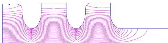
Figure 1: Electric field contour lines of the operating  $\pi$  mode
