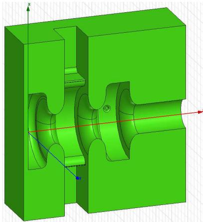
Figure 2: Cross-section of the SwissFEL RF gun.
