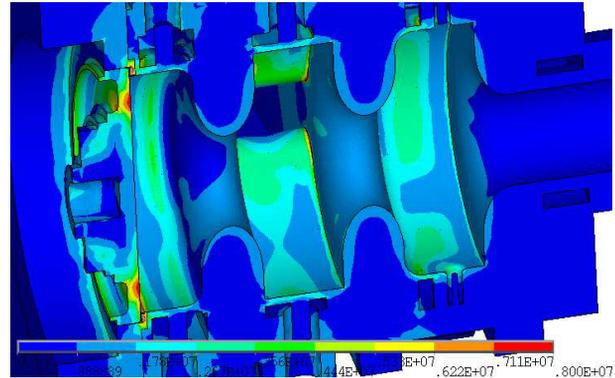
Figure 8: Thermal stress ( $\text{N/m}^2$ ) for a 0.9 kW average load on the SwissFEL RF gun body.
