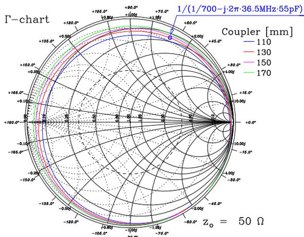
Figure 4: Calculated input impedance without the tetrode shown in a Smith chart. Desired impedance  $Z'$  is shown by a blue circle.
