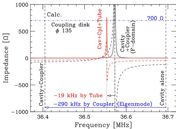
Figure 5: Calculated input impedances for DTL3 with the coupling disk of  $\phi$  135 mm. Black solid and broken lines indicate the real and imaginary impedances, respectively, for the case without the tetrode. Red solid and broken lines denote the real and imaginary impedances, respectively, when the tetrode was attached in parallel as a lumped element.
