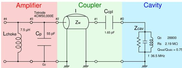
Figure 2: Lumped circuit element diagram of the coupled system of the amplifier, coupler, and cavity of DTL3.
