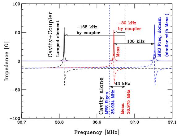
Figure 3: Input impedance for 50 Ω-coupler calculated by lumped circuit element. The real and imaginary parts of the input impedance are shown by solid and broken lines, respectively. The measured values are shown by red lines.
