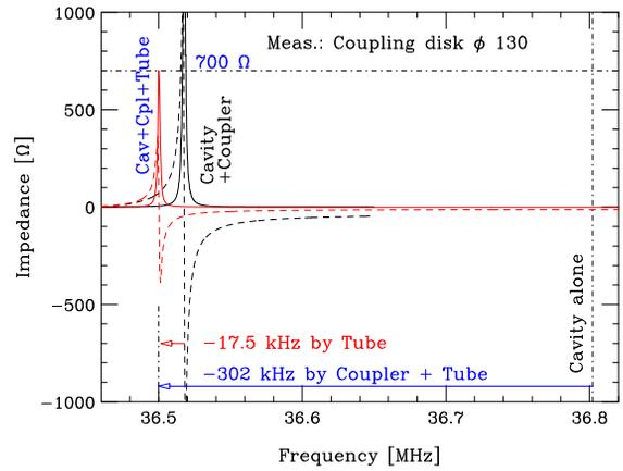
Figure 6: Measured coupling impedances for DTL3 with the coupling disk of  $\phi$ 130 mm. The notation is the same as that in Fig. 5.
