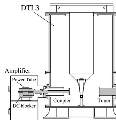
Figure 1: Schematic of the amplifiers coupled to cavity of DTL3. The output from the amplifier is directly connected to the coupler through a capacitor (DC blocker).
