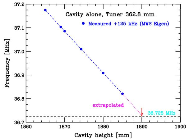
Figure 7: Measured resonant frequency of DTL3 with a movable shorting plate. The frequency shift caused by a removal of the shorting plate ( $0.125$  MHz) is taken into account.
