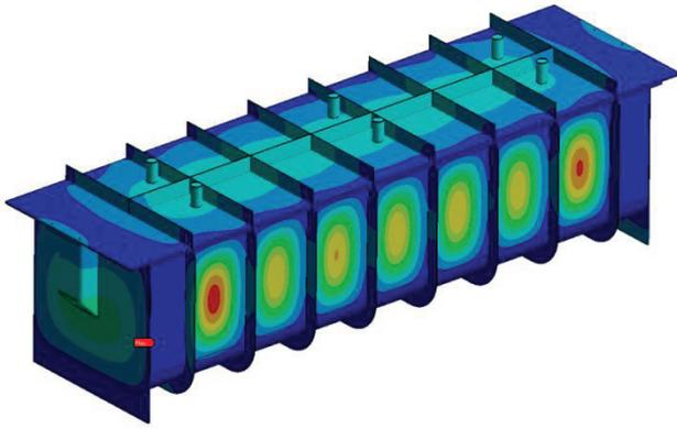
Figure 1: ANSYS results of the vacuum vessel deformation due to a 14.7 psi static pressure gradient across the walls. The red color corresponds to displacements greater than 0.6 inches with the maximum being 0.67 inches.
