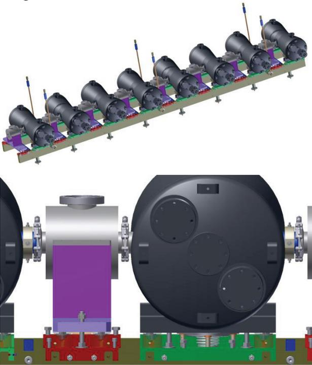
Figure 2: (Top) A cavity/solenoid string mounted on a strong-back. (Bottom) A close up of the alignment hardware for a solenoid and a cavity. The runners move transversely by adjusting two screws which push and two screws which pull (screws not shown but threaded holes they mate with are). One of each adjustment type is on each corner. The runners can be moved up and down by adjusting two vertical screws and placing shims between it and the strong-back.
