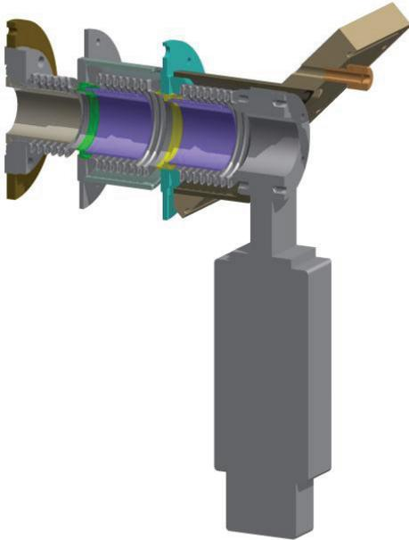
Figure 5: Cross section view of the beam-line gate valve. The total heat leak to 2 K in this design is  $< 0.05$  W. For the 4 K cryomodules the final bellows segment on the left will be removed.
