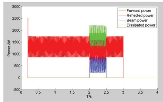
Figure 8: Power needed in ADRC without piezo-tuner. RF power is turned on at  $t=0.2s$  and off at  $t=3s$ . PI without piezo-tuner consumes similar RF power.
