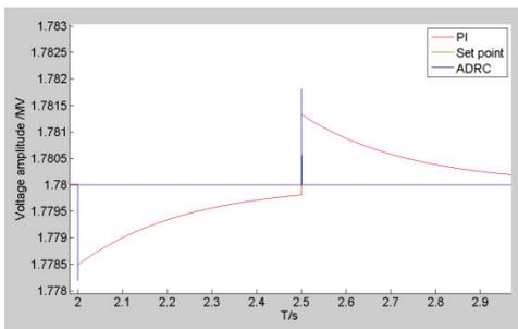
Figure 3: Cavity voltage amplitude fluctuation to reject beam loading. Amplitude's set point (1.78MV) is overlap with blue line.
