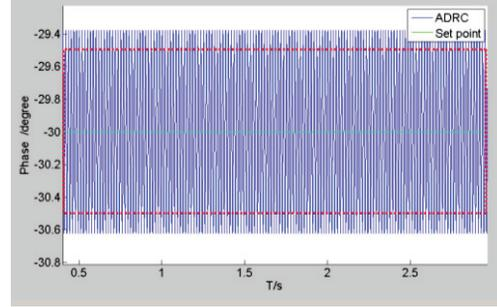
Figure 1: Phase fluctuation to reject microphonics by the original ADRC scheme. The red line marks the fluctuation limit due to stability concern of cavity phase. Microphonics amplitude is assumed to be 20Hz in this calculation.
