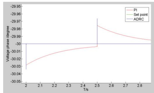
Figure 4: Cavity voltage phase fluctuation to reject beam loading. Phase set point ( $-30^\circ$ ) is overlap with blue line.
