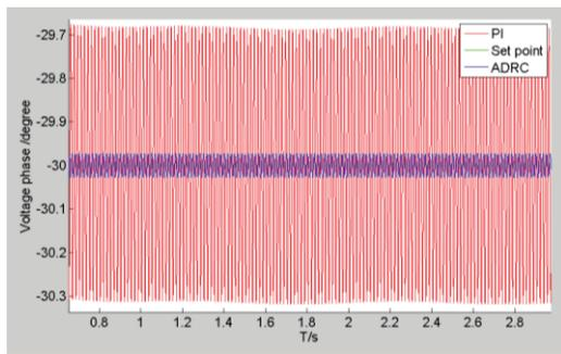
Figure 6: Cavity voltage phase fluctuation for microphonics. Green is set point=-30°.
