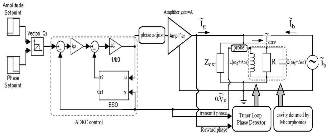
Figure 2: Model of ADRC control with new vector-control scheme
