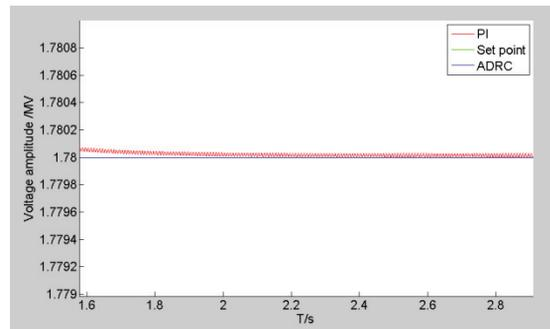
Figure 5: Cavity voltage amplitude fluctuation for microphonics. Amplitude's set point (1.78MV) is overlap with blue line.
