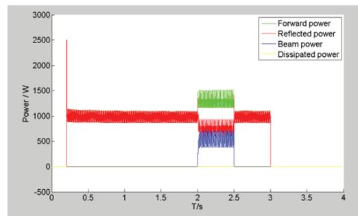
Figure 9: Power needed in PI with piezo-tuner. RF power is turned on at  $t=0.2s$  and off at  $t=3s$ .
