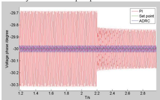
Figure 7: Phase fluctuation reduced by piezo-tuner. Piezo-tuner response time is set to 0.5 ms. Blue is ADRC without piezo-tuner, red is PI with a piezo-tuner turned on at 2.2 s.
