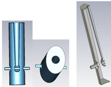
Figure 1: Mechanical model of the elliptical cylinder outer conductor QWR for the structural analysis.
