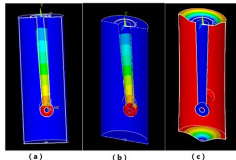
Figure 5: The lowest three vibration modes for stiffened-ring with radius 60mm QWR cavity.
