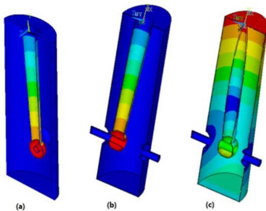
Figure 3: The lowest three vibration modes for the new-shaped naked QWR cavity.
