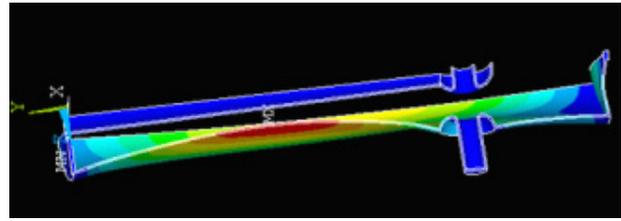
Figure 8: Deformation of ring-and-supporting-rods-stiffened-and-thickened QWR by external pressure:  $df/dP \sim 11$  Hz/mbar.
