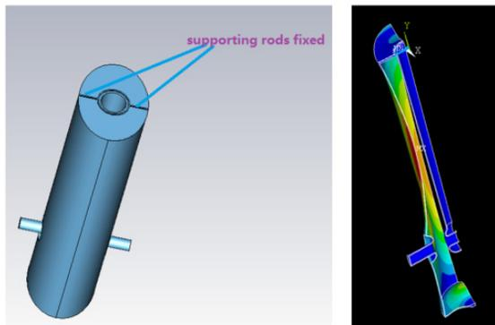
Figure7: Supporting rods on the short plate (left); deformation of ring-and-supporting-rods-stiffened QWR by external pressure:  $df/dP \sim 29$  Hz/mbar.
