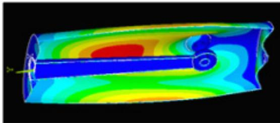
Figure 6: Deformation of ring-stiffened QWR caused by the external pressure, the frequency shift  $\Delta f$  due to the change in ambient pressure  $\Delta P$ :  $df/dP \sim 37$  Hz/mbar.
