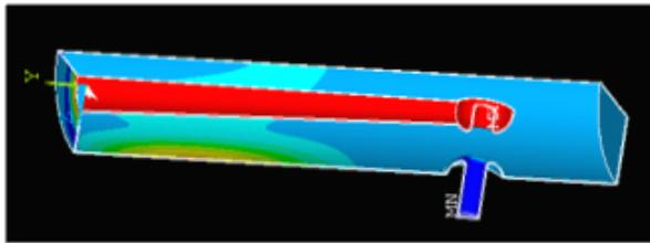
Figure 2: Deformation of the elliptical cylinder outer conductor QWR caused by Lorentz force.
