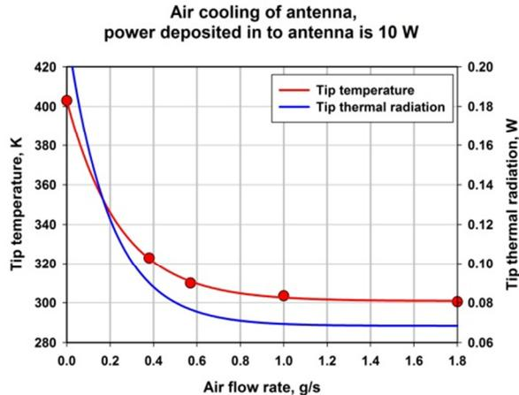
Figure 5: Antenna air cooling, case of 10 W deposition into antenna (325MHz, 30kW, TW).  $\sim 0.3$  g/s flow rate provides acceptable temperature of antenna tip. Thermal radiation at this point  $\sim 0.1$ W
