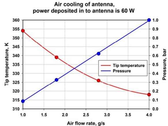
Figure 6: Antenna air cooling, case of 60 W deposition into antenna (650MHz, 120kW, TW).  $\sim 2.5$ g/s flow rate and  $\sim 0.5$  bar pressure provide acceptable temperature of antenna tip. Thermal radiation at this point  $\sim 0.1$ W
