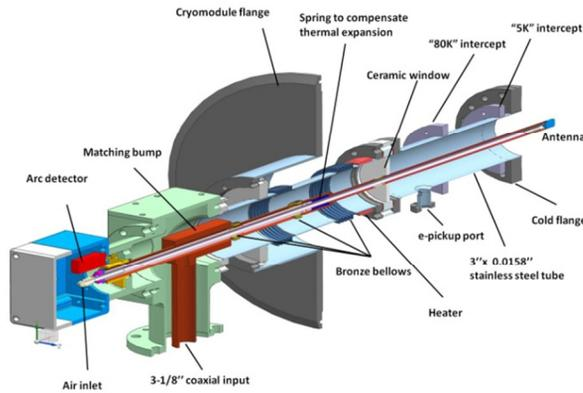
Figure 2: Cut view of 325 MHz coupler.
