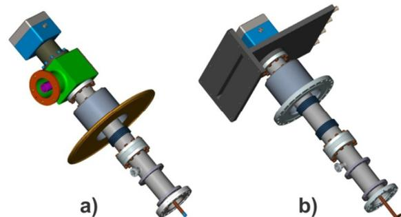
Figure 1: General view of a) 325MHz and b) 650 MHz couplers
