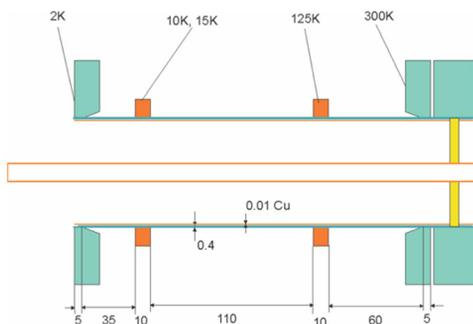
Figure 3: Scheme of vacuum part of coupler which was used for calculation of thermal properties.
