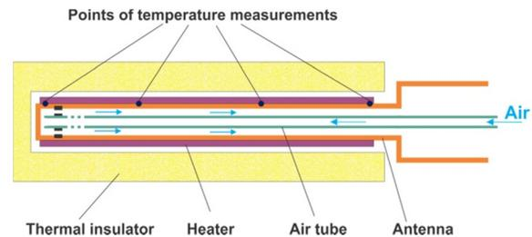
Figure 4: Scheme of measurements of antenna air cooling effectiveness.
