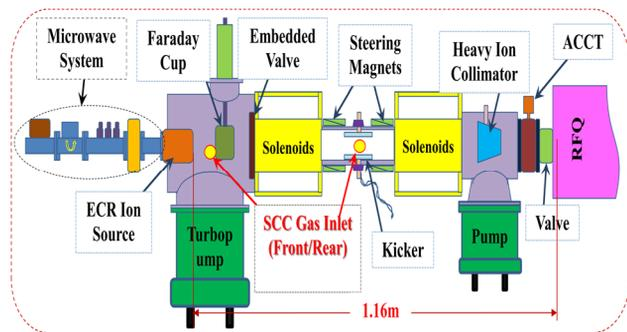
Figure 3: Schematic view of the helium injector.
