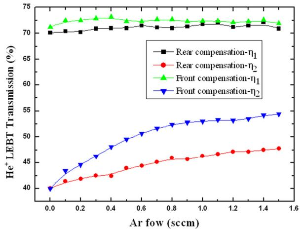
Figure 2: LEBT transmission of 30keV/65mA He<sup>+</sup> beam with front compensation and rear compensation.
