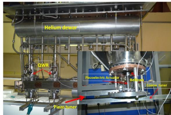
Figure 2: The piezoelectric actuator based mechanical tuner in third linac cryo module along with close view.
