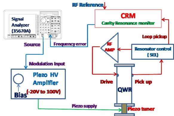
Figure 4: Set up for measurement of frequency response or piezoelectric based mechanical tuner.
