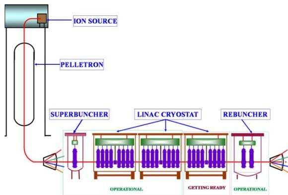
Figure 1: The schematic of IUAC linac.
