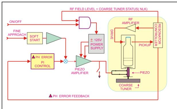
Figure 6: Block diagram of Piezoelectric close loop control scheme.
