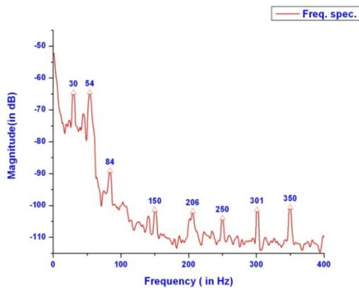
Figure 3: All the resonant modes of the resonator in linac cryostat.
