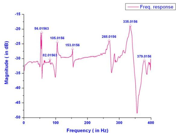
Figure 5: Frequency response of the piezoelectric tuner.
