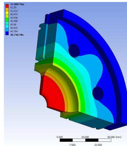
Figure 6: Temperature distribution in a disk of the C-band structure for a 40 °C inlet water temperature.
