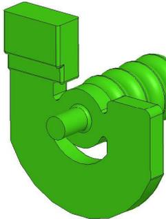
Figure 5: 3D computer model of the J-type coupler.
