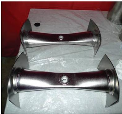
Figure 3: Spoke bars after welding.
