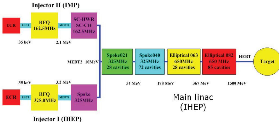
Figure 2: Layout of ADS accelerator
