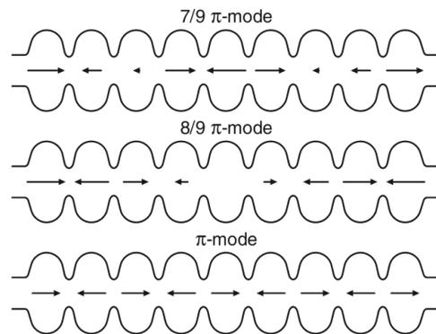
Figure 1: Sketch of electrical field  $\vec{E}_z$  distribution along the axis for the acceleration and the two next fundamental modes of Tesla type cavities [1]
