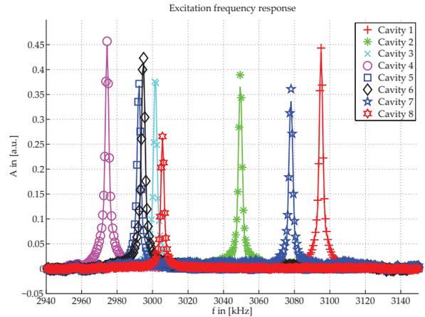
Figure 3: Individual cavity response to a sweeping sinusoidal excitation around 3 MHz, comp. Fig 2
