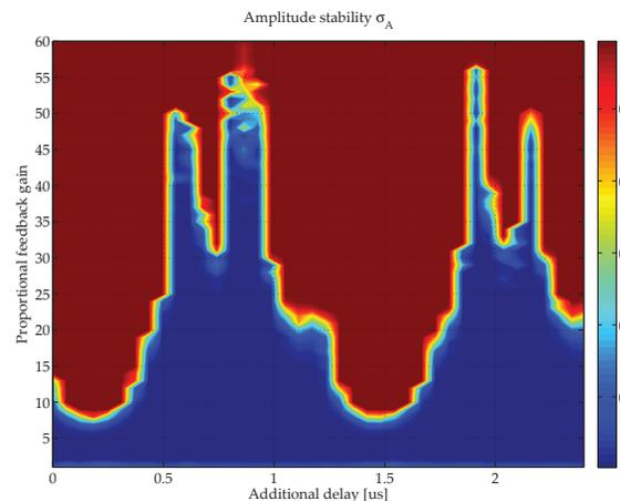
Figure 4: Stability diagram for scanning the amplitude error as function of feedback gain and additional loop delay
