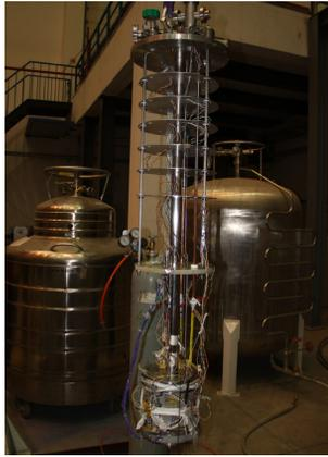
Figure 8: Assembly of test insert for CADS solenoid
