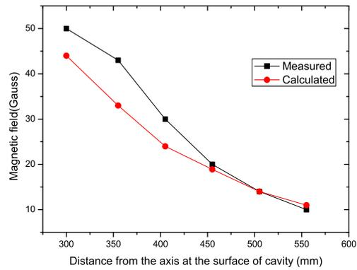
Figure 11: Comparison between the measured fringe field and the calculated value
