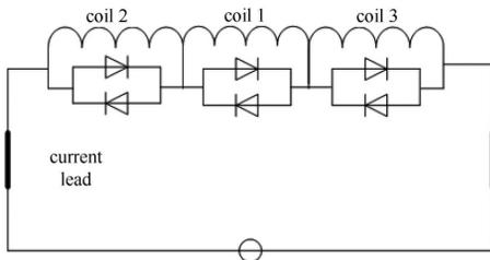
Figure 9: Quench protection circuit
