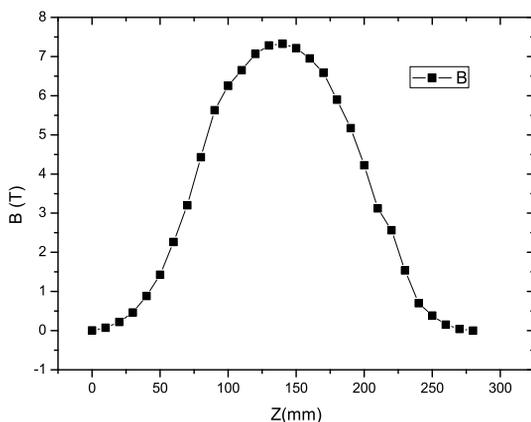
Figure 10: The measured magnetic field distribution along the axis of the solenoid
