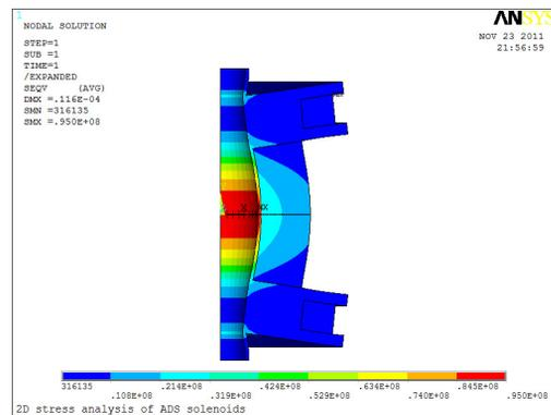
Figure 7: Simulated stress distribution of the solenoid caused by the electromagnetic forces
