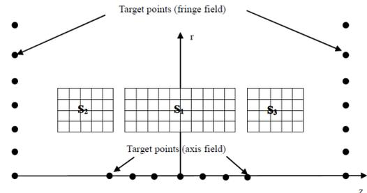
Figure 2: The feasible coil regions with numerical grid.
