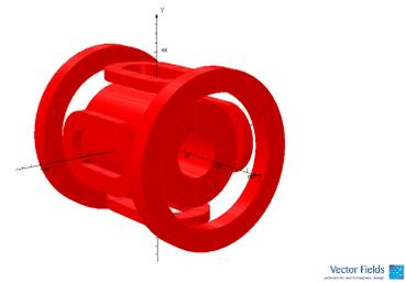
Figure 5: Coils configuration of CADS solenoid
