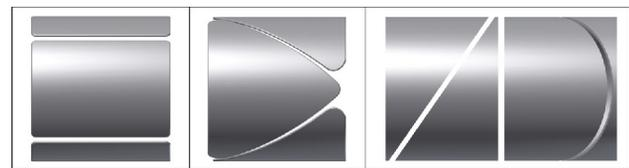
Figure 3: Side views of the three X-Y steerer configurations studied: (left) parallel quartered cylinder, (middle) diagonally quartered cylinder, and (right) two sets of diagonally halved cylinders.
