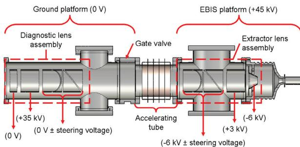
Figure 2: The electrostatic model of the I-E beamline. Nominal component voltages are shown for the injection cycle and are referenced to their respective platforms.
