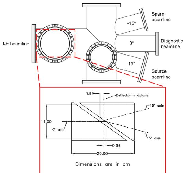
Figure 4: The electrostatic switchyard configuration and deflector positioning necessary to achieve an injected beam on the  $0^\circ$  beamline axis.
