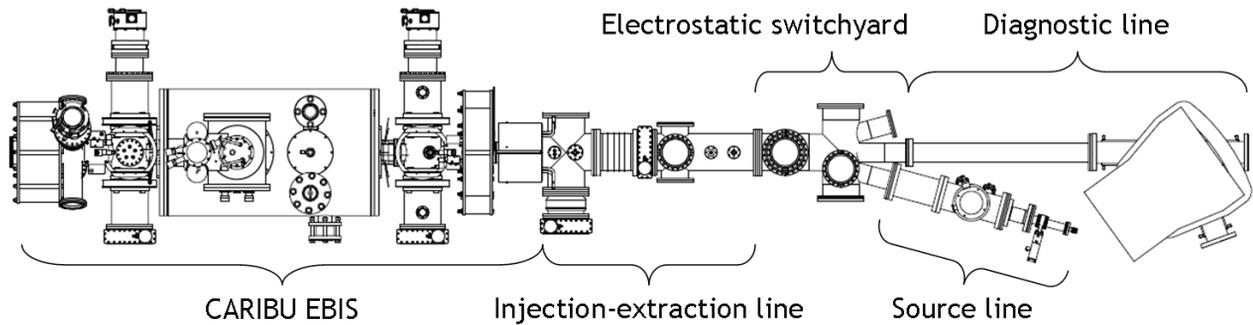
Figure 1: The layout of the EBIS charge breeder and transport lines for offline testing.
