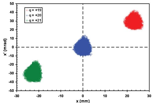
Figure 5: The transverse phase space distributions of  $^{133}\text{Cs}^{+19}$ ,  $^{133}\text{Cs}^{+20}$ , and  $^{133}\text{Cs}^{+21}$  at the entrance to the Faraday cup after the analyzing magnet.
