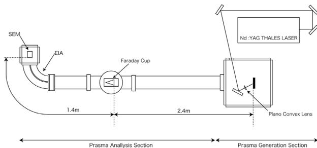
Figure 3: Plasma analysis beam line.
