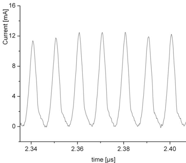
Figure 8: Bunched structure after the RFQ.
