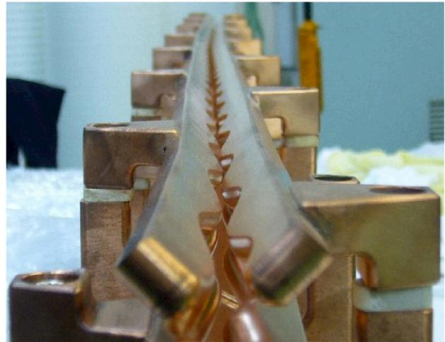
Figure 1: Deformed vanes.
