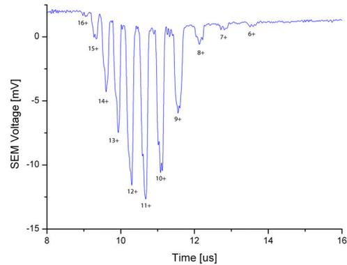
Figure 4: Detected signal by secondary electron multiplier.
