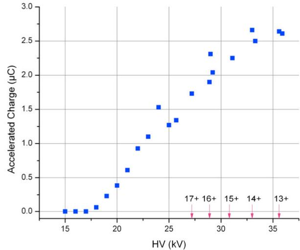
Figure 9: Accelerated charge vs. injection voltage.
