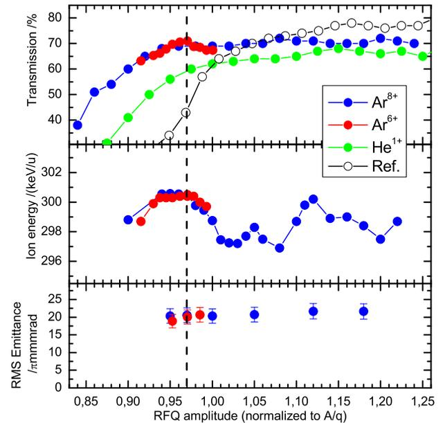
Figure 1: Beam commissioning results (top to bottom): Transmission, ion energy and beam emittance for different ions as a function of the rf amplitude, normalized to the mass-to-charge ratio. Reference data: Old RFQ; dashed line: Derived working point.
