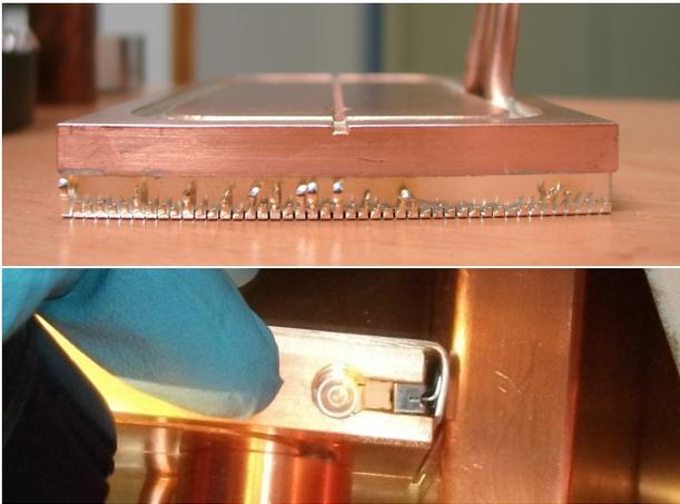
Figure 2: Tuning plate with burnt contact springs (top) and new contacts (bottom). The thick silver foil is pressed against the stem by spring steel foil and steel wedges.
