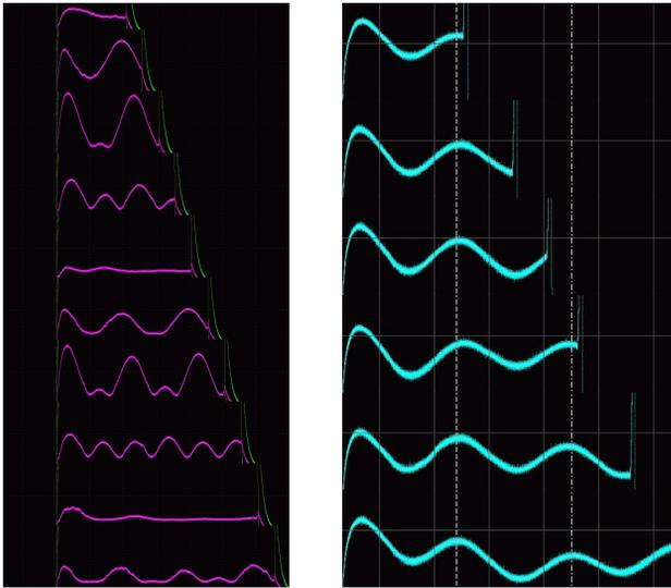
Figure 5: Rf signal modulation at 50 Hz (reflected power, left) and 1 Hz (phase difference forward/reflected, right) pulse repetition rate for pulse lengths of appr. 2-6 ms.
