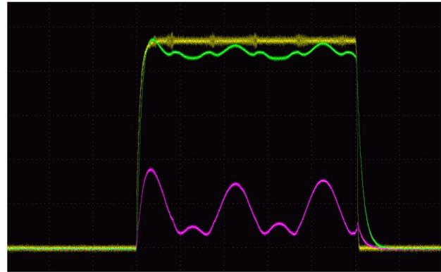
Figure 3: Modulation of the rf tank signals. Magenta: Reflected power; green: Forward power; yellow: Tank amplitude (read out).
