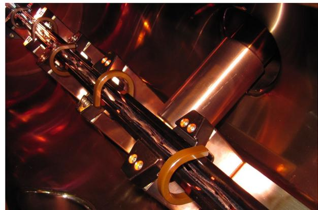
Figure 4: RFQ structure with mounted Vespel clamps. A plunger is moved in from the top right corner.
