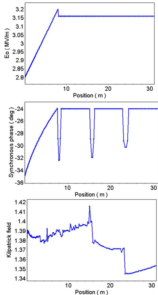
Figure 1: Design E0, synchronous phase and Surface field, along the DTL.
