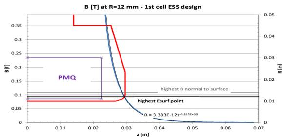
Figure 4: fringe magnetic field in the first cell of tank1.
