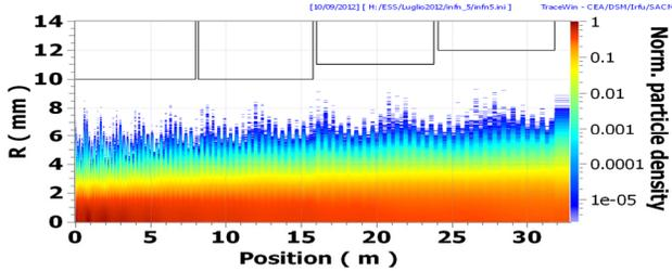
Figure 3: Particles density along the DTL.
