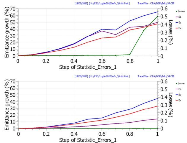
Figure 7: Losses (green) and emittances as a function of applied error on quads, with (bottom) and without (top) steerers.
