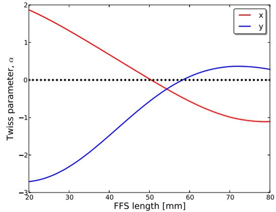
Figure 6: Twiss parameter  $\alpha$  as a function of the FFS length.
