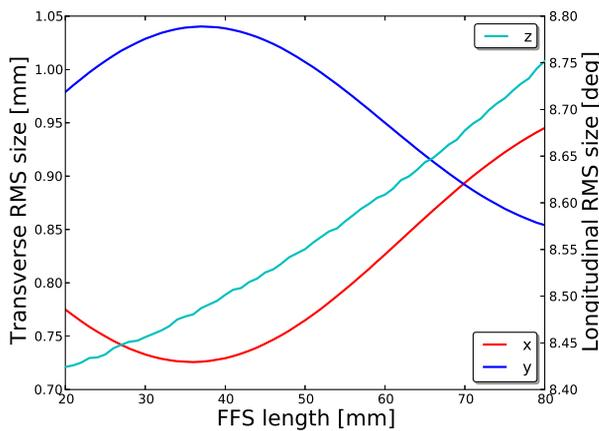
Figure 5: Beam size as a function of the FFS length.
