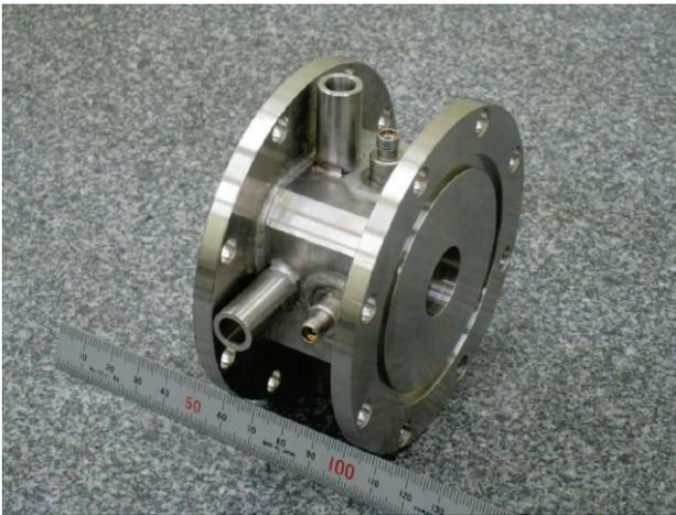
Figure 3: Fabricated BPM for linac.
