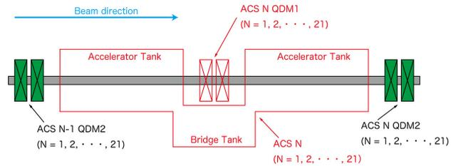
Figure 2: Layout of the quadrupole array in A0BT.
