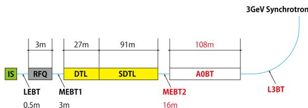
Figure 1: Diagram of the J-PARC linac.
