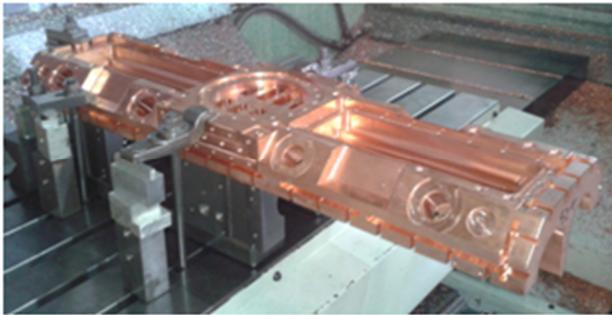
Figure 7: RFQ vane being manufactured.
