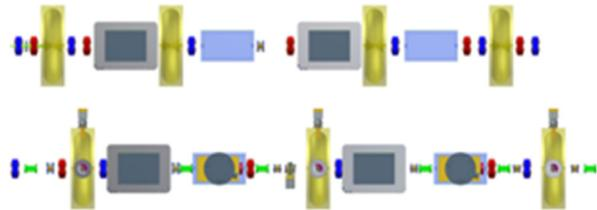
Figure 8: Schematic MEBT baseline layout (top) and a proposed alternative design (bottom).
