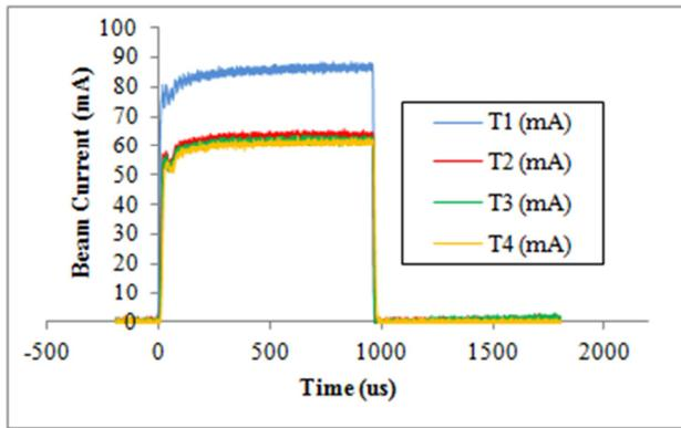
Figure 2: 1 ms beam current profiles at 50 Hz, at different positions: ion source (T1), inside the LEBT (T2, T3) and LEBT output (T4).
