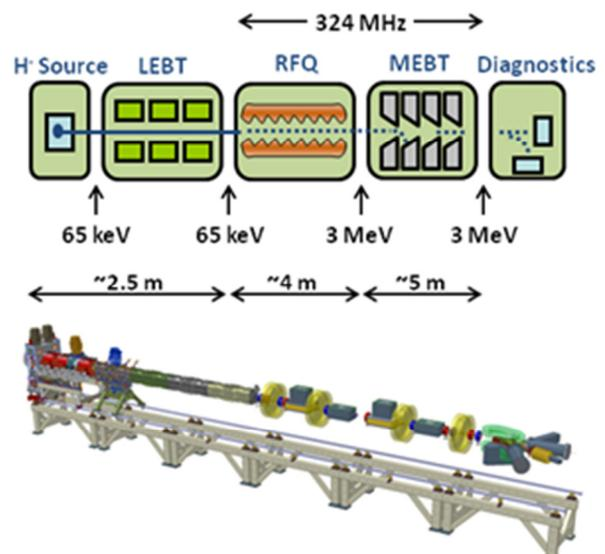
Figure 1: Schematic FETS layout.
