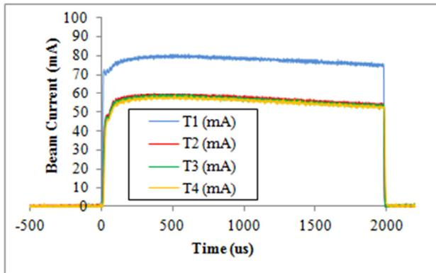
Figure 3: 2 ms beam current profiles at 25 Hz.
