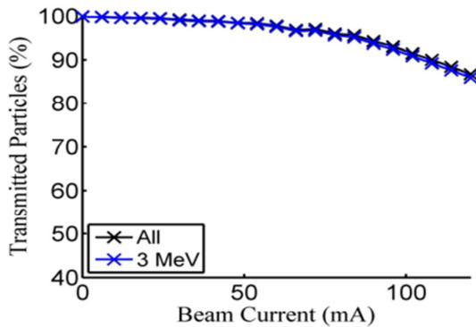
Figure 6: RFQ beam transmission.
