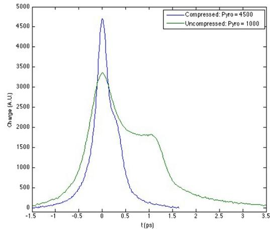
Figure 2: Preliminary results for longitudinal bunch profiles as measured by the xTCAV. Shown are two bunch profiles for the maximally compressed bunch (blue) and an uncompressed bunch (green).
