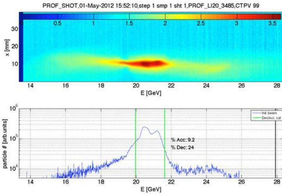
Figure 4: Image from cherenkov spectrometer from beam after passing through lithium vapor. Approximately a quarter of the bunch has interacted with the plasma and lost energy and just under 10% has gained energy.
