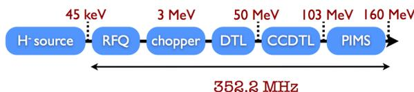
Figure 1: Linac4 block diagram.
