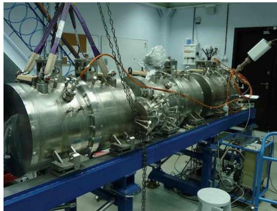
Figure 4: CCDTL module during vacuum test at BINP, Novosibirsk.
