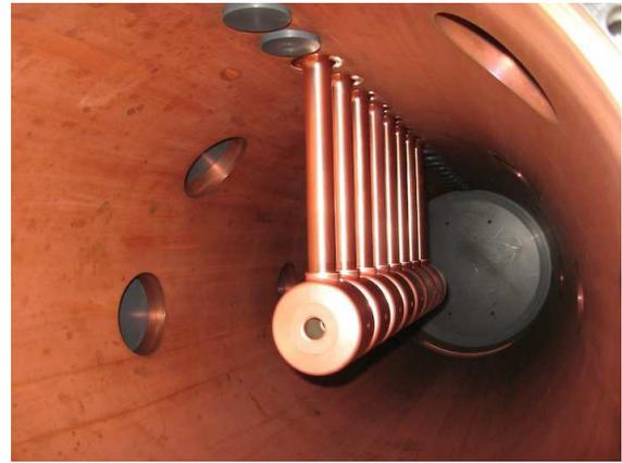
Figure 3: First segment of the first DTL tank.
