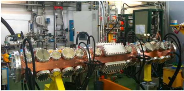
Figure 2: Completed Linac4 RFQ in the 3 MeV test stand.
