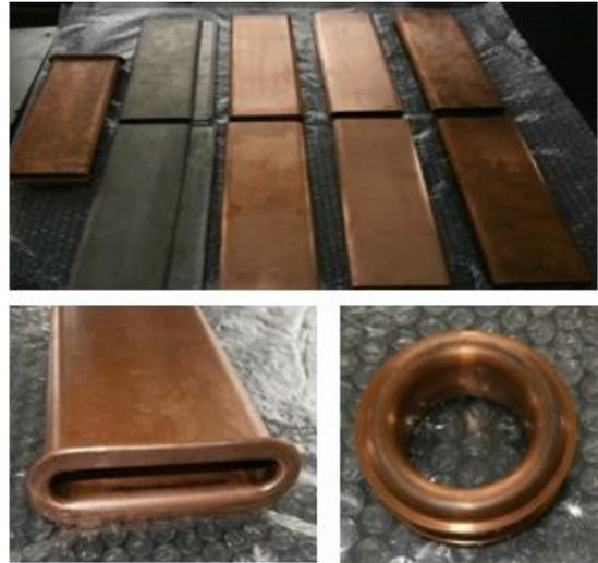
Figure 8: Parts of copper CH cavity.
