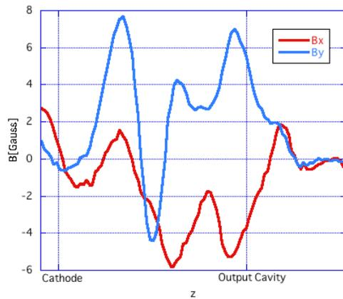
Figure 7: The measured transverse magnetic fields.
