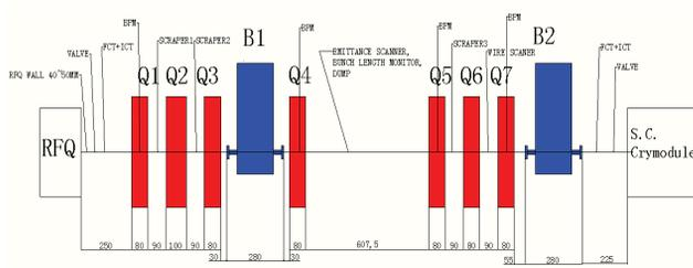
Figure 5: Layout of beam diagnostics in MEBT.
