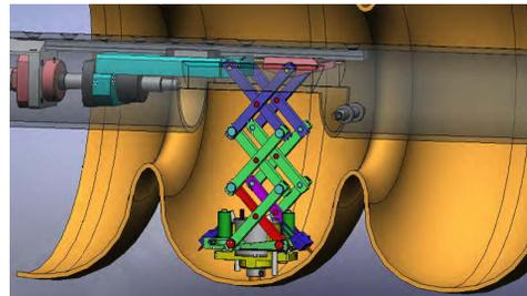
Figure 13: The grinding head assembly that has a tiny monitoring camera protrudes by a motor control towards the area to be treated.
