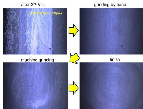
Figure 14: The progresses on the local grinding effect. The defect detected by the optical inspection was removed by the treatment.
