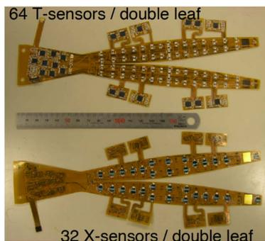
Figure 6: Leaf shaped flexible PCB.
