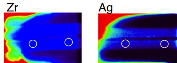
Figure 12: Obtained radiography images for targets of Zr and Ag. Both target materials give better visibility for the defects (sputter balls on the surface).
