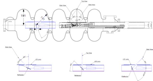
Figure 1: CavCam3 in SPL cavity.
