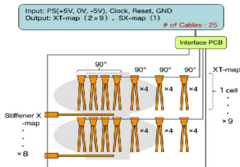
Figure 5: The inter-connection for the XT-map system.
