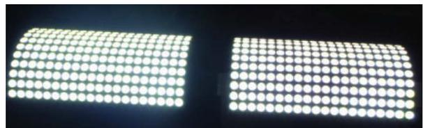
Figure 4: All the LED's are lighted. A diffusing panel will be install on the LED's to form the light strip. 14 chips/line x 2 lines/strip x 10 strips/side x 2 sides = 560 chips are used.
