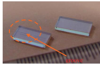
Figure 2: Field Enhancement groove machined in a planar diamond sample.
