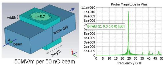
Figure 1: Left: geometry of the diamond resonator: length = 4mm, width = 1.2mm, beam gap = 4mm and overall width = 8mm. Right: spectrum of the wakefield (simulation).
