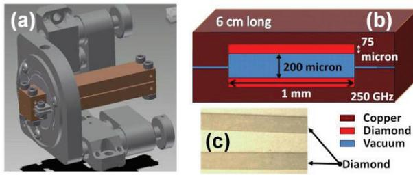
Figure 4: (a) 250 GHz structure mounted on a positioning holder; b) structure dimensions; c) photo of diamond after the experiment exhibiting no visible damage.
