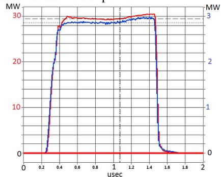
Figure 10: Input (red) and Output (blue) RF power waveforms
