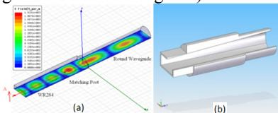
Figure 7: Mode converters with matching post (a) and rectangular-to-round transition (b)
