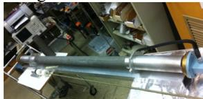
Figure 8: TE11 mode RF load under low power test
