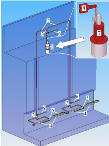
Figure 1: Original RF setup of the SLAC linac; 1 is XK-5 Klystron, 2 is WR284 Waveguide Branches, 3 is Power Dividers, 4 is Accelerating Sections, 5 is High Power RF Loads, 6 – Low Power RF Loads
