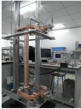
Figure 3: Vertical cold RF test for the 1.1m C-band traveling accelerating structure.
