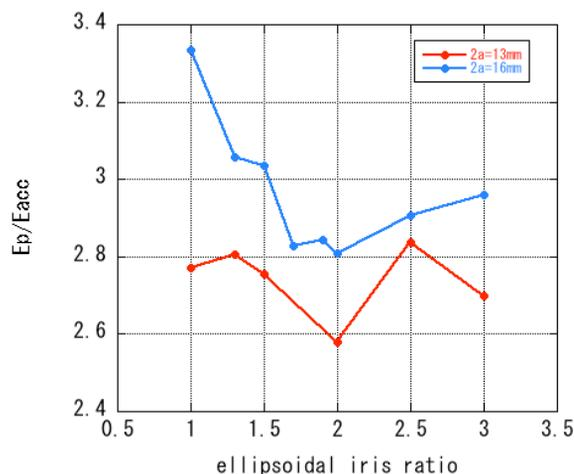
Figure 4: Ratio of maximum surface electrical field to the on-axis electric field ( $E_p/E_{acc}$ ) depending on the ratio of B/A.
