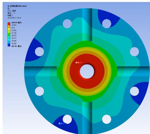
Figure 5: Temperature distribution of the accelerating structure in 120 pps operation
