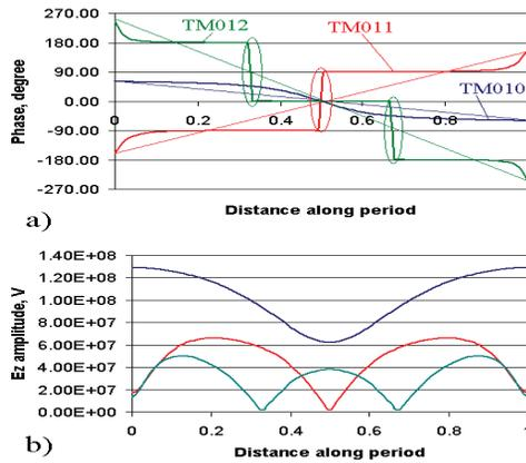
Figure 3: Phase (a) and amplitude distributions along DLW cell axis for the first ( $\Theta = 120^\circ$ ), the second ( $\Theta = 320^\circ$ ) and the third ( $\Theta = 510^\circ$ ) passbands.
