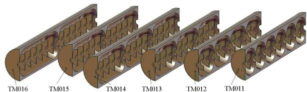
Figure 6: Structures with washers in DLW cells.
