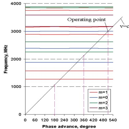
Figure 8: Dispersion diagram of DLW with washers,  $TM_{02}$ -like operating mode in the cell,  $\Theta = 510^\circ, m$  - number of azimuthal variations.
