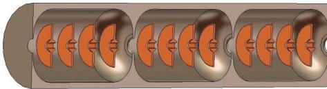
Figure 7: The structure with washers and drift tubes in DLW cell.
