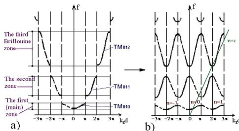
Figure 1: DLW dispersion diagram formation for  $TM_{01}$  wave.
