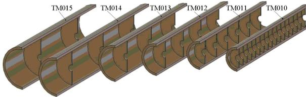
Figure 4: The relative DLW cells dimensions for operation in the first and in higher  $TM_{01}$  passbands.
