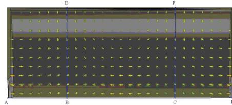
Figure 5: Electric field of  $TM_{012}$  mode in DLW cell.
