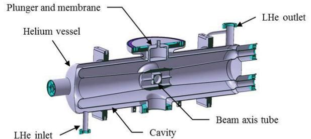
Figure 1: the IFMIF HWR prototype.
