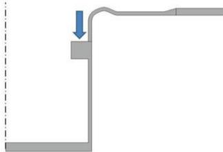
Figure 6: geometry of the niobium plunger. The arrow represents the force applied by the actuator.
