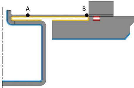
Figure 3: thermal loads on the 2D axis symmetrical model: in blue, the convection with the liquid helium, in orange, the RF losses, in red, the seal dissipation.
