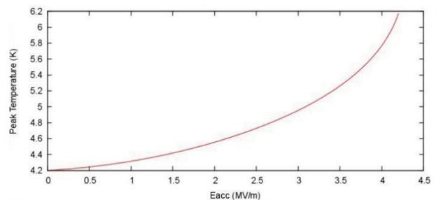
Figure 5: peak temperature of the membrane versus the accelerating field in the cavity (no dissipation in the seal).
