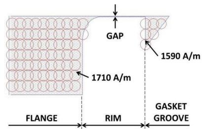
Figure 4: 2D simulation results of the influence of the gap between the membrane and the flange of the cavity on the gasket (H-field values are given for 4.5 M/m, the nominal accelerating field).
