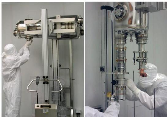
Figure 4: Clean room assembly for the 72 MHz QWR's.
