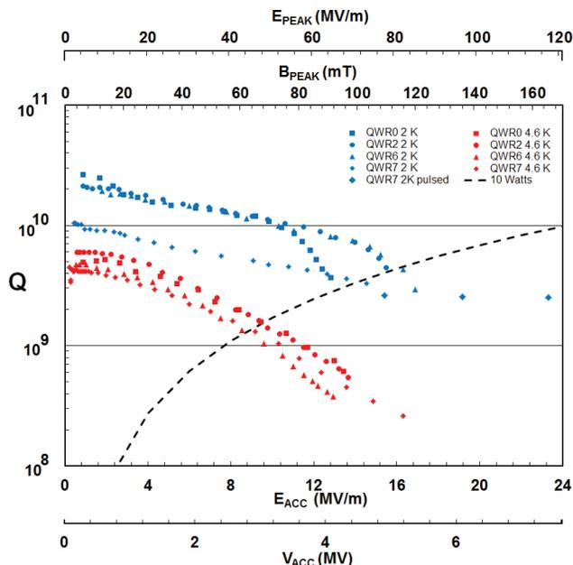
Figure 2: Quality factor versus accelerating gradient, voltage and surface fields at 2 and 4 K ( $l_{eff}=\beta\lambda=0.32$ m)
