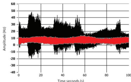
Figure 5: Microphonic amplitude reduction in a quarter-wave cavity due to centering the central conductor
