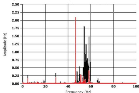
Figure 6: Fourier spectrum for data in previous Figure. Microphonics are lower (red) but the mechanical Q remains high when no mechanical damper is used.
