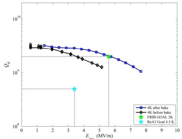
Figure 4:  $Q_0$  versus  $E_a$  showing improvement in cavity performance after low temperature bakeout application.
