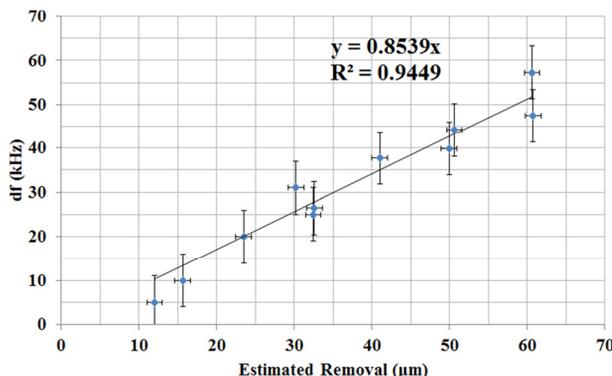
Figure 3: Measured frequency shift (kHz) versus the estimated material removal (microns).
