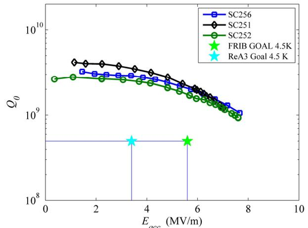
Figure 7:  $Q_0$  vs.  $E_{acc}$  at 4K for ReA3  $\beta=0.085$  QWRs
