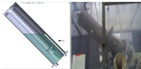
Figure 2: Differential etching setup for removal in high electric field region of the  $\beta=0.085$  to increase frequency.
