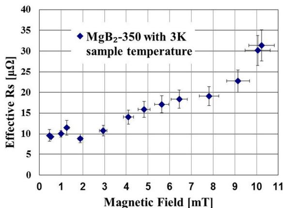
Figure 5: Effective surface resistance of MgB<sub>2</sub>-350 versus magnetic field at 3 K.
