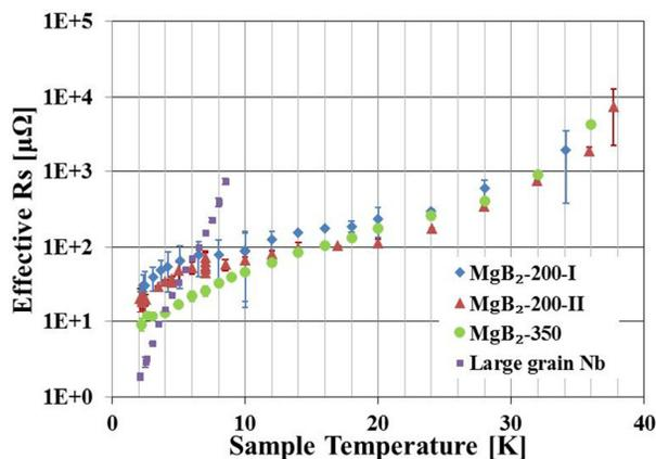
Figure 4:  $\blacklozenge$  MgB<sub>2</sub>-200-I  $\blacktriangle$  MgB<sub>2</sub>-200-II  $\bullet$  MgB<sub>2</sub>-350 Effective surface resistance of MgB<sub>2</sub> on sapphire substrate  $\blacksquare$  Surface resistance of large grain Nb sample.
