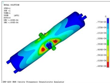
Figure 2: Structural analyses results of HWR with beam pipes fixed (cavity deformation).
