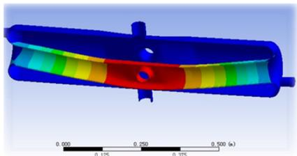
Figure 5: One of Model analyses results of HWR cavity with cleaning pipes free ( cavity deformation).
