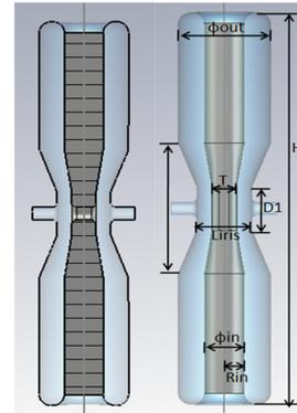
Figure 1: The cross section of HWR cavity with the main geometric parameters: Liris-iris to iris length, T-inner conductor thickness, D1-cavity diameter.
