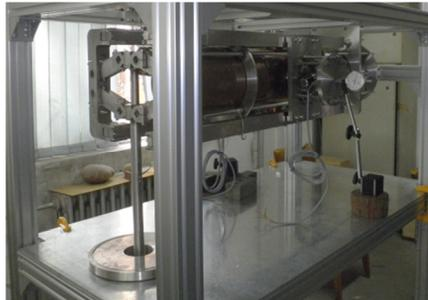
Figure 7: Mechanical Tuner of HWR cavity test with copper HWR prototype .
