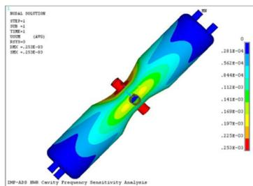
Figure 3: Structural analyses results of HWR with beam pipes free (cavity deformation).
