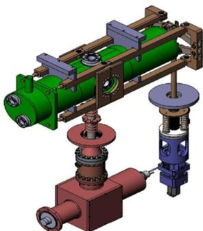
Figure 6: The IMP mechanical tuner: tuner(dark gray), helium vessel (green), and coupler (red).
