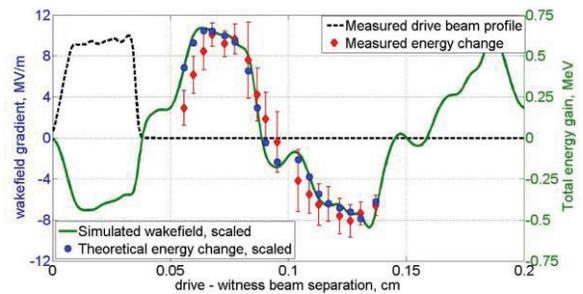
Figure 5: Energy gain of the witness beam as a function of separation from the drive beam.
