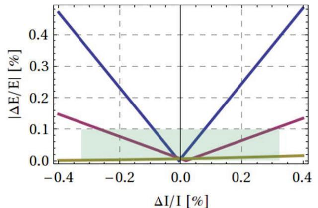
Figure 2: Total energy deviations at the end of the linac with corresponding intensity changes in the linac: blue line - stable injector, purple line - stable linac and yellow line - stable energy. The parts of the lines lying in the shaded area satisfy the stability goal.
