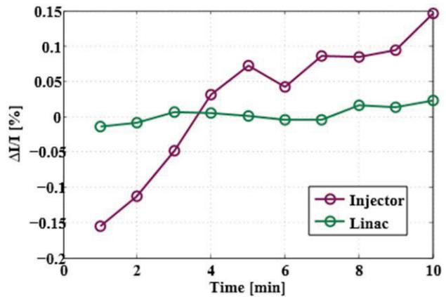
Figure 4: Illustration of the stabilization of the intensity in the linac by adjusting the intensity in the injector.
