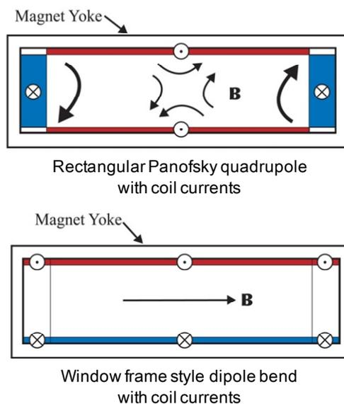
Figure 4: Quadrupole and Dipole Current Flows [7].
