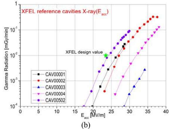
Figure 5: Cold RF test results: after surface preparation at DESY: (a) –  $Q_0(E_{acc})$ , (b) – X-ray( $E_{acc}$ ).
