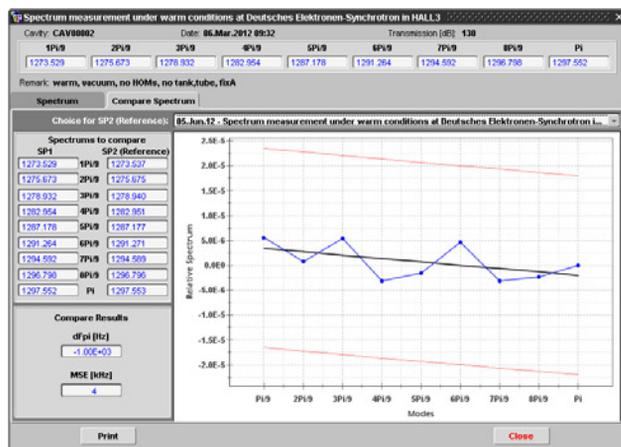
Figure 4: Comparison of two spectra (two columns at the left panel) for CAV00002. RS – blue broken line.
