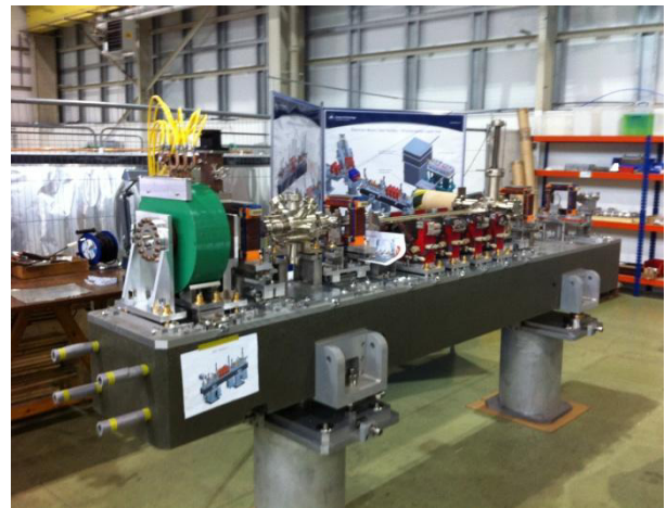
Figure 6: EBTF photoinjector in the assembling stage.
