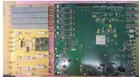
Figure 3: RF front-end (left) and digital processing board (right)
