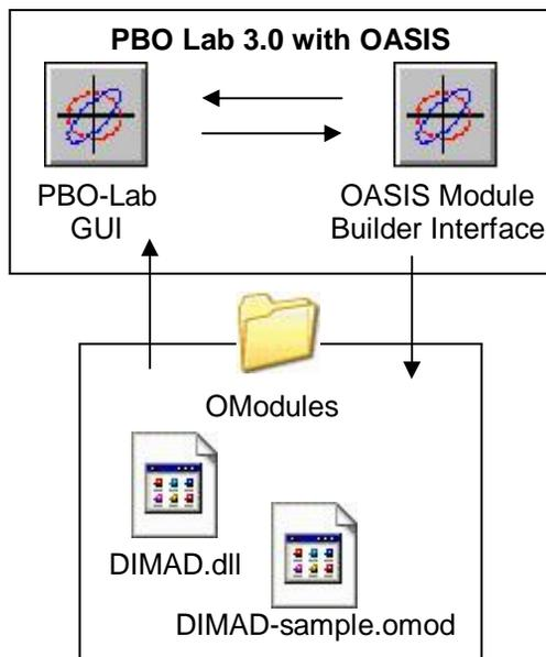
Figure 2: Application Modules can be interactively developed and executed in the Module Builder Interface and exported for use directly in the PBO Lab GUI as (.omod) OModule definition files.
